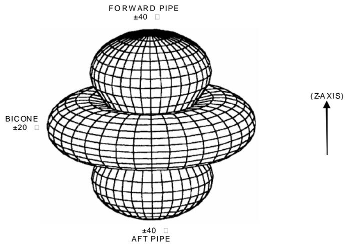
**Figure B-4. DIRECTV KU-79W Wide Beam TT&C Antenna Coverage**
