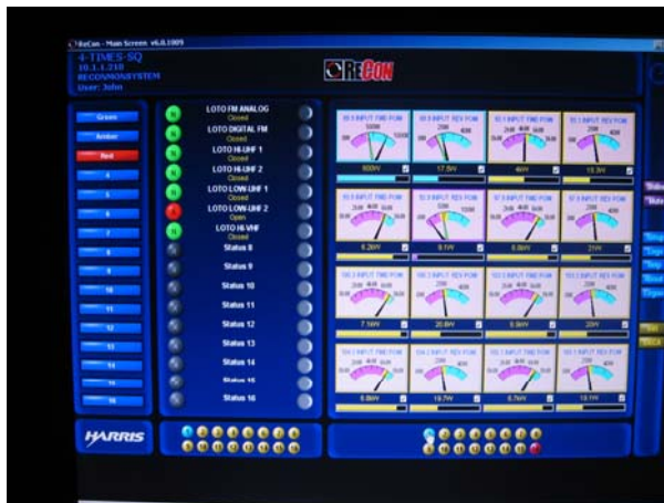
Figure 12. CRT display of the Harris RECON™ system used for continuous monitoring of the status of each transmitter at the 4TS facility. Trip points may be set to cause activation of alarms based on transmitter power levels.
