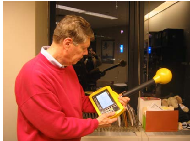
Figure 7. Using the Narda SRM-3000 portable spectrum analyzer and isotropic antenna to document RF field level in a building adjacent to the 4TS site.
