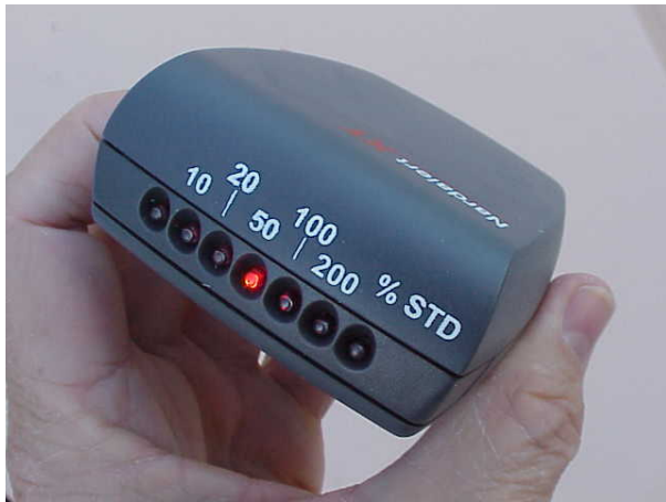
Figure 9. The NardAlert™ personal monitor detects RF emissions and weights the field intensities in accordance with the FCC MPE. The alarm threshold may be set at user selected values as a percentage of the MPE. The device also indicates the greatest field to which it has been exposed and a history of the monitor field readings can be downloaded to a personal computer for further analysis. The unit detects RF fields across the frequency range of 100 kHz to 100 GHz.
